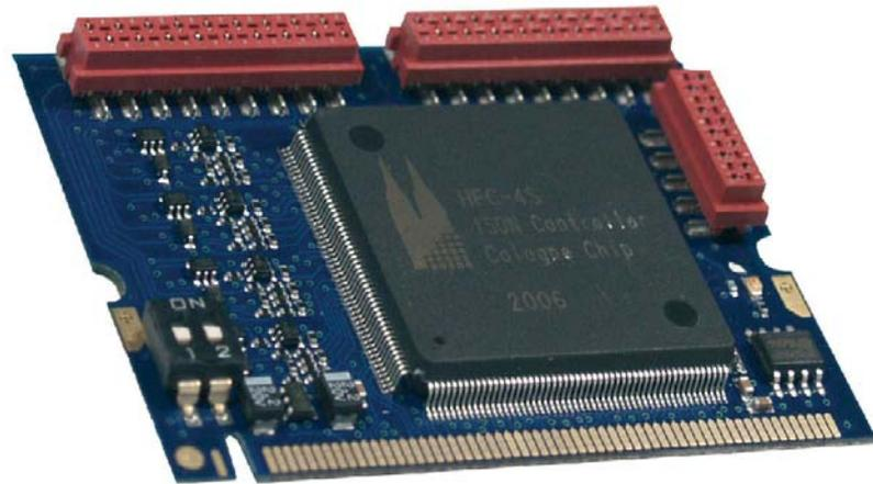
Application 1: Integration of an ISDN PBX    Application 2: Voice over IP gateway for BRI
